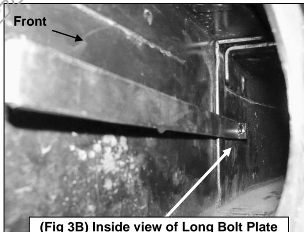
(Fig 3B) Inside view of Long Bolt Plate installed in driver side frame channel
